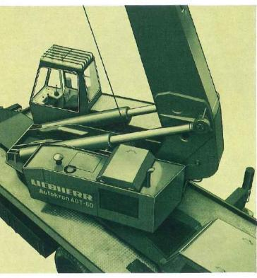
The crane is mounted on a four or six-wheel LIEBHERR chassis with front-wheel steering. With the crane lowered down for transportation, the 165-hp water-cooled diesel engine gives the unit a maximum road speed of 60 km/hour.
